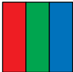
Figure 9.1 An LCD colour pixel is spatially multiplexed into three subpixels. At a suitable viewing distance, light from the subpixels is summed by the viewer's visual system.
