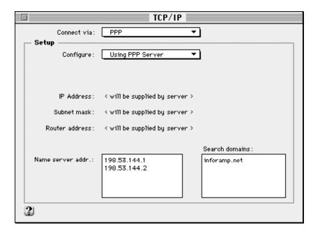
Open the TCP/IP control panel to obtain this dialog. At the top of the panel, choose *PPP*. I have an Ethernet interface on my machine, so I am presented with a few other choices; you may have only AppleTalk (MacIP) and PPP. Set *Configure* to *Using PPP Server*. Set the *Name Server Addresses* to the IP addresses of your ISP's domain name servers. Set *Search Domains* to the domain name of your ISP. When you close the panel, you will be invited to save the configuration.
